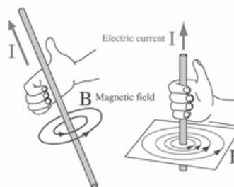
**Magnetic Fields and The Current Loop:** Any coil of wire will produce a magnetic field as illustrated below. A series of coil will produce a uniform magnetic field within the coil itself. The Left Hand and Right Hand rules apply with exception that the fingers will indicate the flow of negative or positive charge respectively, and the thumb will indicate the direction of the magnetic field ( $B$ ).
