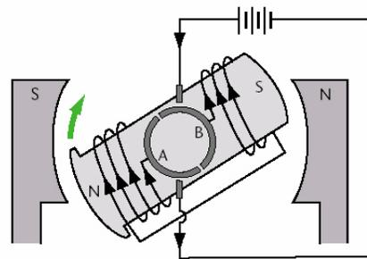
As the armature continues to rotate, the force of attraction between the north pole of the armature is attracted to the south pole of the external magnetic field and the entire cycle starts over again (see diagram 5).
