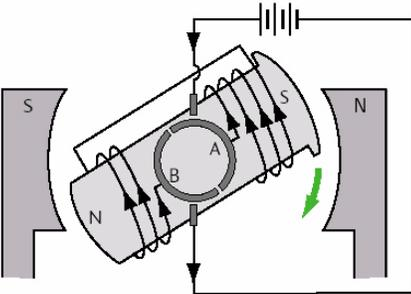
In the second diagram, the current is flowing from A to B through the armature. Using the RHR (Right Hand Rule), a south pole is generated at the end of the coil closest to point A. The force of magnetic repulsion causes the armature to rotate counter clockwise.
