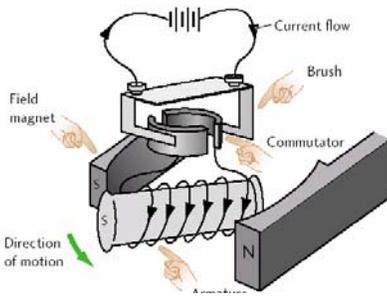
As discussed earlier, electricity through a conductor or a coil will induce a magnetic field. This phenomenon is exploited in the electric motor. Observe the diagrams of the basic motor design below.
