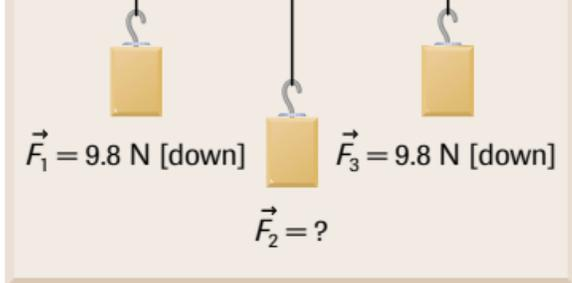
The above diagram shows a possible setup for a vertical force board. (You may prefer to modify the setup, however, using a force table instead of a force board, as suggested for this activity.) In this vertical force board, there are three different forces, each acting on a different string. If two of the forces are known, the third force can be determined. Describe how you would determine the unknown force  $\vec{F}_2$ .
