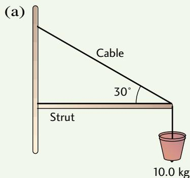
22. In problem 21, how much horizontal force must the strut provide?
