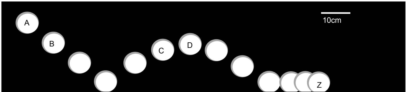
assume the strobe was flashing at 20Hz. Remember  $f = \frac{1}{T}$  so  $T = \frac{1}{f}$ . This gives us a time interval between flashes of  $T = \frac{1}{20} = 0.05s$ . From this, you can determine the speed of the object at various times
